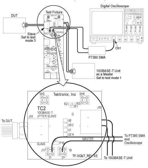
Note: When using high input impedance differential probe, ensure that each of the single ended lanes is terminated with 50  $\Omega$ .
