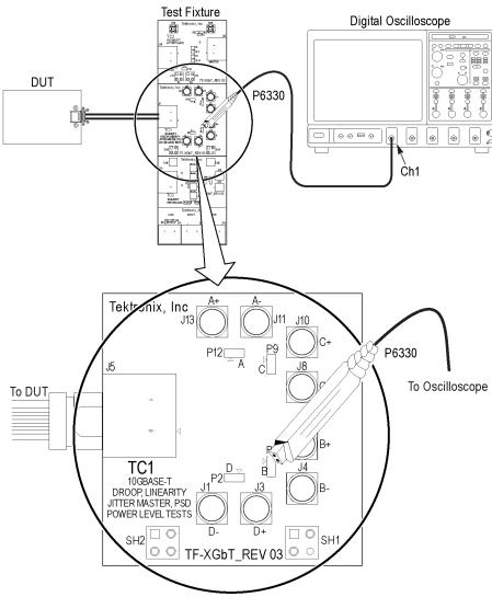
Note: When using high input impedance differential probe, ensure that each of the single ended lanes is terminated with 50  $\Omega$ .
